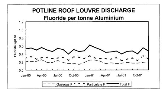
The following graph shows the average total plant fluoride per tonne aluminium during 2000 and 2001.
