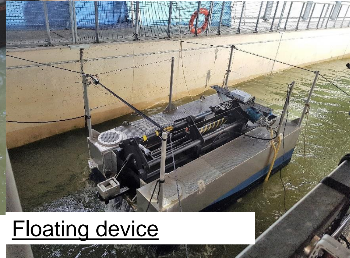
OWC w. hydroturbine
