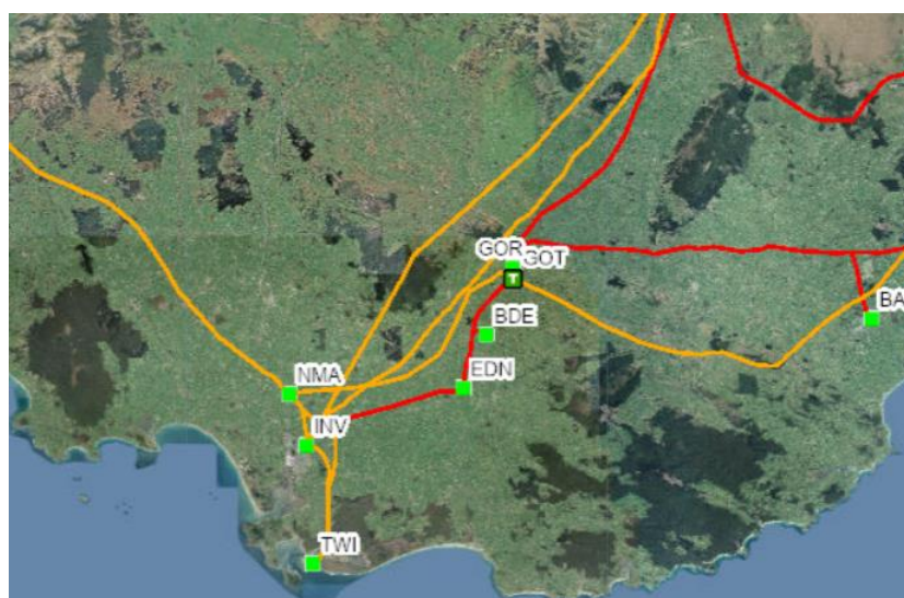
Map 1: The transmission network in Southland and Southern Otago; the yellow lines illustrate the 220 kV network, and the red lines illustrate the 110 kV network. It includes our Grid Injection Points and Grid Exit Points in Southland; (Manapouri (MAN), North Makarewa (NMA), Invercargill (INV), Tiwai (TWI), Edendale (EDN), Brydone (BDE), Gore (GOR) and the Gore Tee (GOT).
